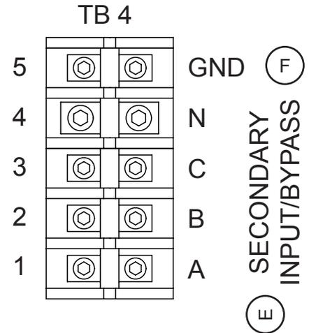
FIGURE 9.5 – 15-30KVA POWER CABLING LUGS
