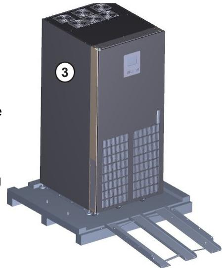
5. Place the tie brackets in the slots at the upper and lower ends of the ramps.
