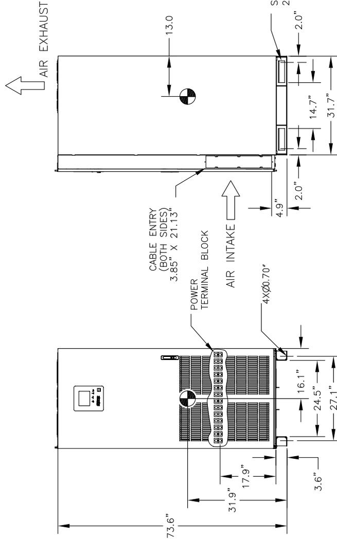
FIGURE A.4 – 4400 80 KVA PHYSICAL DIMENSIONS
