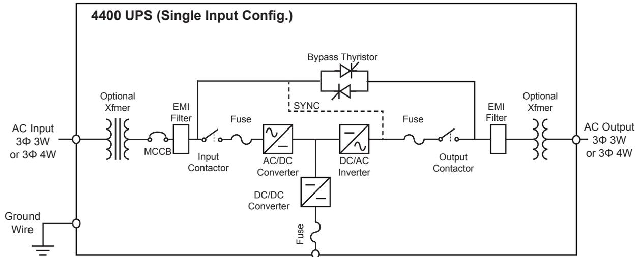
**FIGURE 9.1 – 4400 SINGLE INPUT ONE-LINE DIAGRAM**
