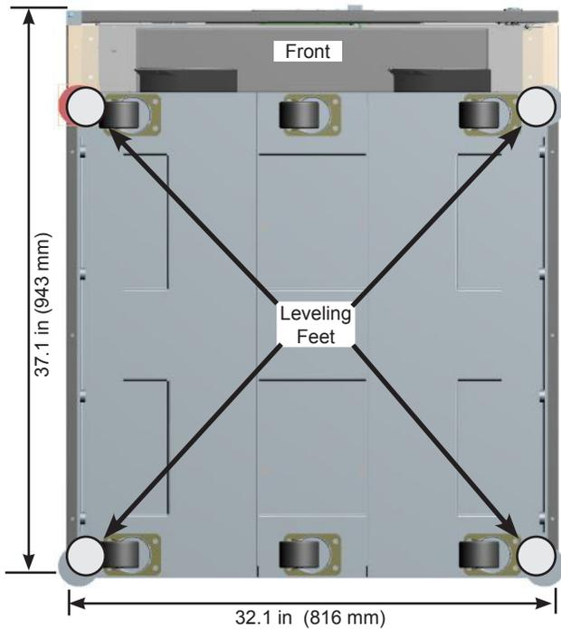
**FIGURE 8.5 FOOTPRINT FOR 50 KVA USING LOAD LEVELING FEET**
