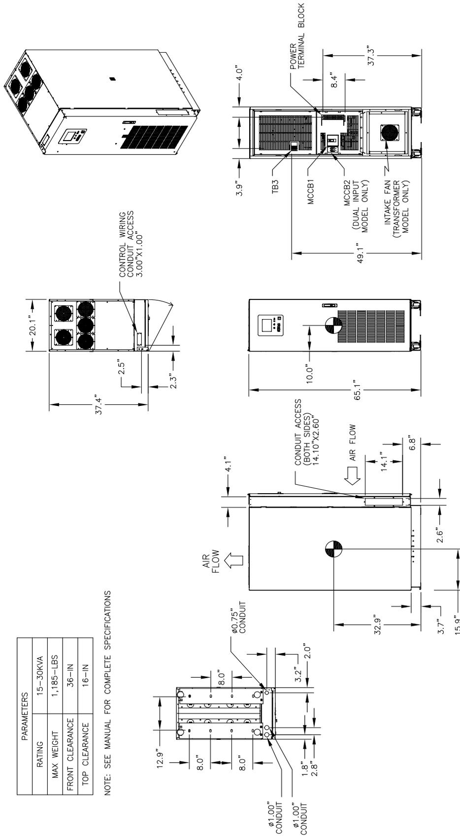
FIGURE A.1 – 4400 15-30 KVA PHYSICAL DIMENSIONS
