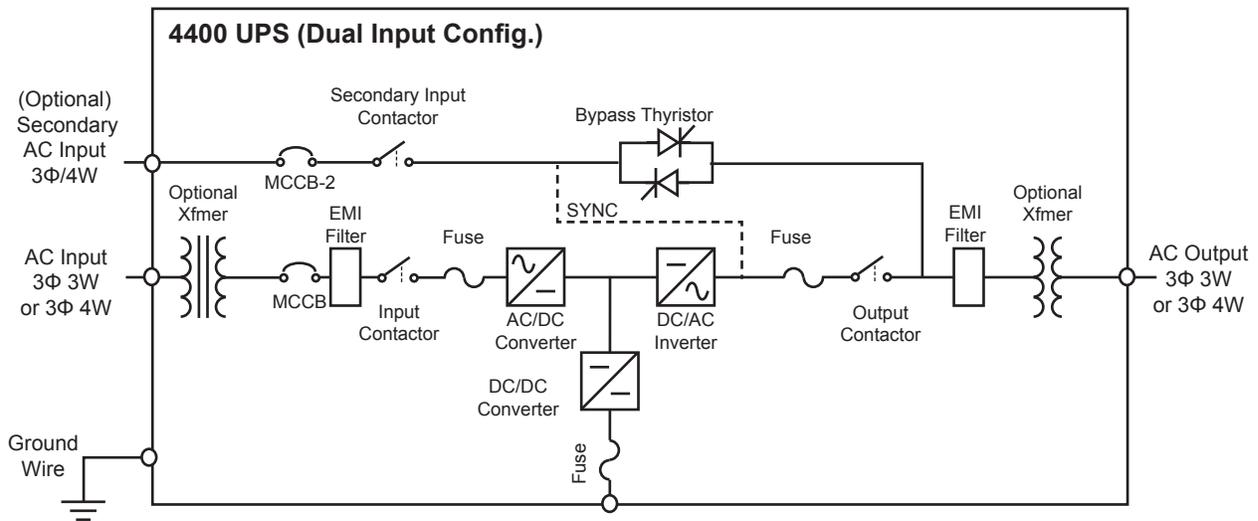
**FIGURE 9.2 – 4400 DUAL INPUT ONE-LINE DIAGRAM**
