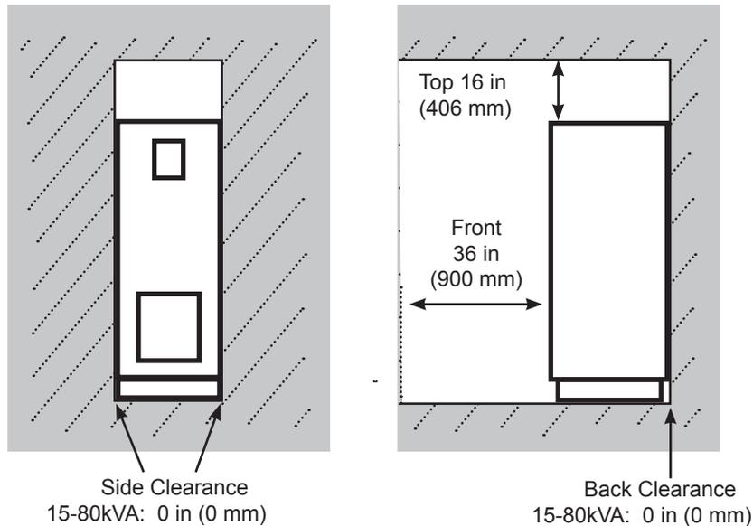
**FIGURE 8.1 CLEARANCE FOR UPS USING LEVELING FEET**
