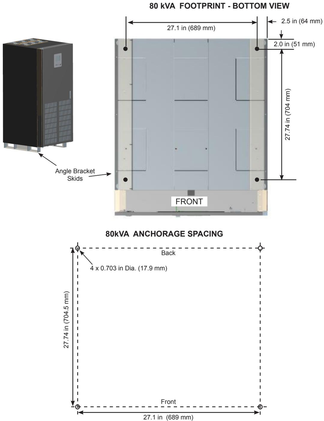
**FIGURE 8.6 ANCHORAGE HOLE LOCATIONS – 80kVA UNITS (Standard)**
